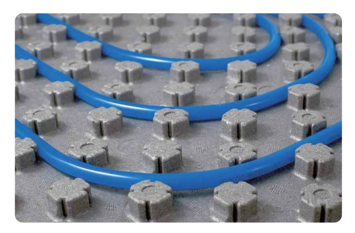
**Super D** is an underfloor heating and cooling system with low thermal inertia and low thickness, characterised by  $\emptyset$  12 mm PB pipe anchored to an insulated base and embedded in the special lowered screed.
