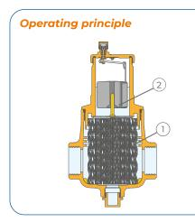
The deaerator uses the combined action of several physical principles. The active part consists of an assembly of concentric metal mesh surfaces (1). These elements create the whirling movement required to facilitate the release of micro-bubbles and their adhesion to these surfaces.
