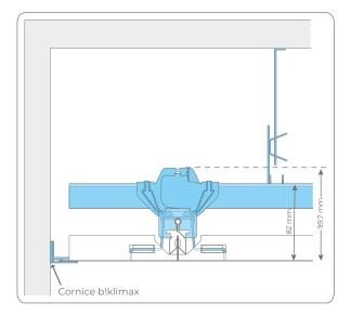
**b!klimax+ Quadrotti HP** metal radiant panels are designed to be installed on the ceiling on a special metal support frame that is suspended and concealed (double continental structure with Winger by Atena S.p.A.).
