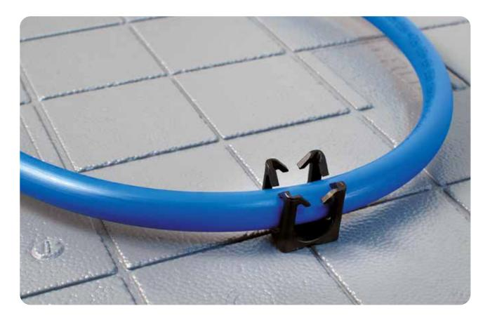
**Smooth Cover HP** is a traditional underfloor radiant heating and cooling system, characterised by pipes anchored to an insulated base by special fixing clips and embedded in the screed.
