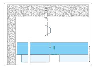
The **b!klimax+ Quadrotti** metal radiant panels are designed to be installed on the ceiling on a T-shaped metal support frame with a 15 mm base that emphasises its three-dimensionality, guaranteeing excellent aesthetic performance of the system. The structure can be equipped with a special "anti-seismic kit" to respond to the safety and stability requirements of the ceiling in all areas with high seismic risk.
