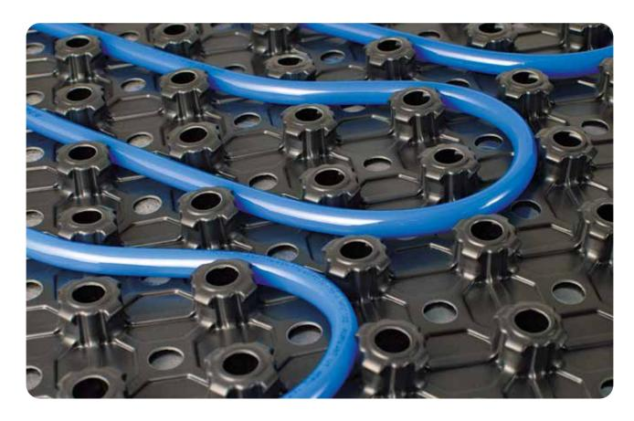
**Zero Level AD** is an underfloor heating and cooling system with low thermal inertia and very low thickness, characterised by  $\emptyset$  12 mm PB pipe anchored to a thermoformed slab and embedded in the self-levelling concrete.
