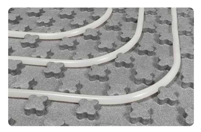
**Super D17** is an underfloor heating and cooling system with low thermal inertia and reduced thickness, characterised by  $\emptyset$  17 mm PE-Xa pipe anchored to an insulated base and embedded in the special lowered screed.
