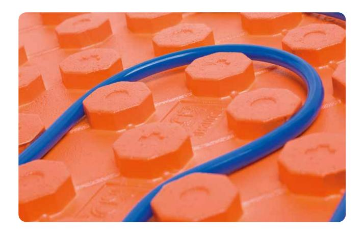
**Acoustic Plus** is a traditional underfloor radiant heating and cooling system, characterised by pipe anchored to an insulated base and embedded in the screed.
