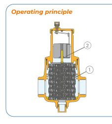
The air separetor uses the combined action of several physical principles. The active part consists of an assembly of concentric metal mesh surfaces (1). These elements create the whirling movement required to facilitate the release of micro-bubbles and their adhesion to these surfaces.
