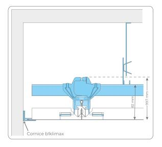
The **b!klimax+ Copper 8** metal radiant panels are designed to be ceiling installed on a special hanging and hidden metal support frame (double structure with Winger by Atena S.p.A.). The use of the patented "Winger" coupling facilitates the assembly and guarantees a perfect installation.
